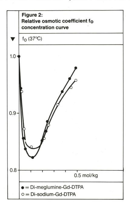
surements the following apparatus was used: Vapour pressure osmometer (Knauer GmbH, Berlin), digital precision densitometer DMA 10 (A. Paar KG, Graz), and automated Ubbelohde viscosimeter (Schott Geräte GmbH). The osmotic coefficients were determined by an isopiestic method with sucrose as the reference substance.<sup>9,10</sup>
