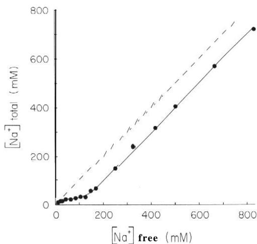
FIGURE 1. The relation between total  $Na^+$  concentration and free  $Na^+$  concentration (measured with the  $Na^+$  selective electrode) in a 10% hemoglobin solution containing increasing amount of NaOH. Dashed line indicates the case where there is no adsorption and all  $Na^+$  present is free.
