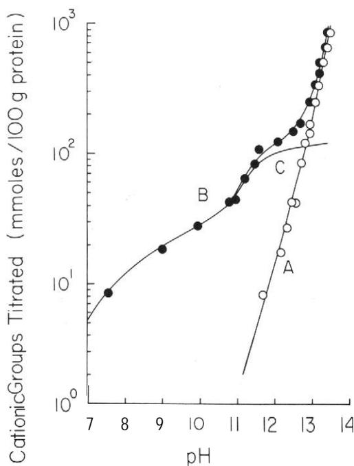
FIGURE 4. Titration curve of 10% hemoglobin (B) and of distilled water (A). The corrected titration Curve C, which was obtained by subtracting Curve A from Curve B, represents OH groups "bound" to hemoglobin at the different pH's.
