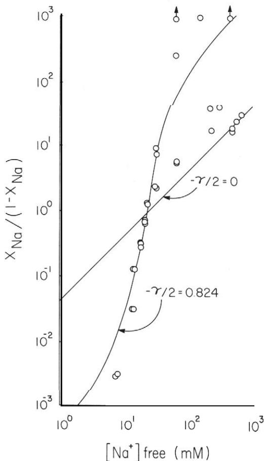
FIGURE 8. Log-log plot of  $\text{Na}^+$  adsorbed on 10% hemoglobin against the concentration of free  $\text{Na}^+$  in the medium. Solid line is a theoretical curve calculated according to Equation 2 with  $K_{x \rightarrow \text{Na}}^{\text{oo}}$  equal to  $4.15 \times 10^2$  and  $-\gamma/2 = 0.824$  Kcal/mole ( $n = 4.09$ ). Straight line is a theoretical (Langmuir) adsorption curve with  $-\gamma/2 = 0$  Kcal/mole ( $n = 1$ ).
